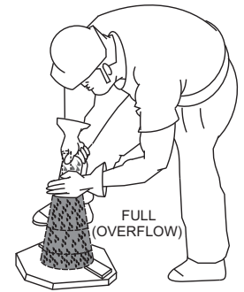
Figure 68-C. Slump Test (Full-Overflow)
